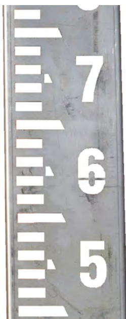
Detail of perforated staff gauge
