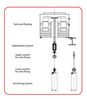
The measuring of the movements of the two pendulums, that is of the wire part of the pendulum, can be performed manuallywith portable removable coordinometer EGS model, or automatically using the different automatic coordinometers produced by us.
